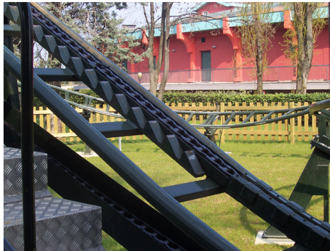
Figure 6: Anti-rollback installed on track
