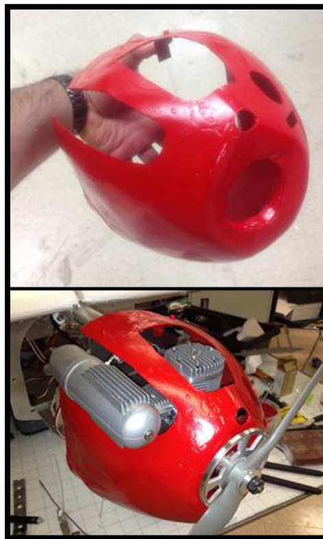
Figure 95 - Final steps of the Cowl manufacturing process
