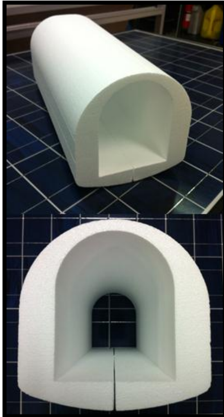
Figure 97 - CNC Foam Cutting of the Body Fuselage
