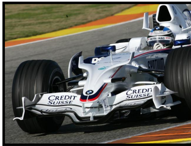
Figure 4 - Front Wing of a Formula 1 Car used to create Down force
