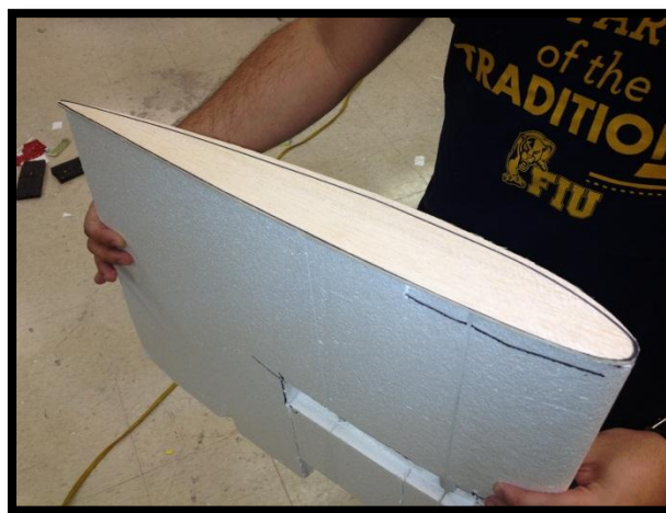
Figure 102 - Balsa wood reinforcement profiles
