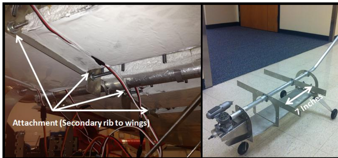
Figure 81 - Secondary Rib Design and Features
