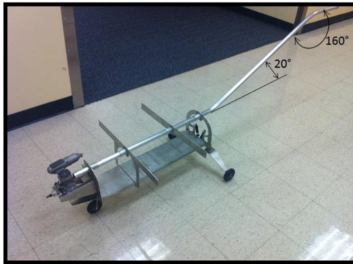
Figure 89 - Bending process of the Aluminum Tube or Backbone
