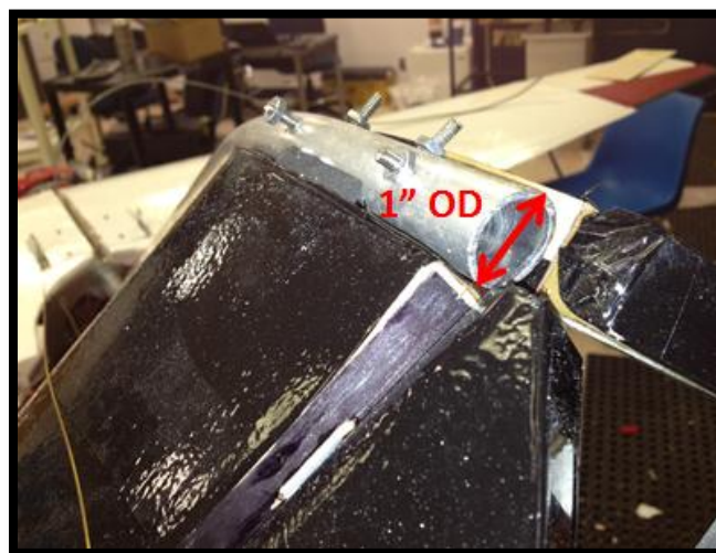
Figure 88 - Backbone or Main Tube Design and Specifications
